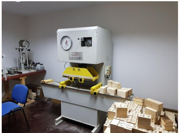
Figure 9: Testing QC machine for glulam samples.
