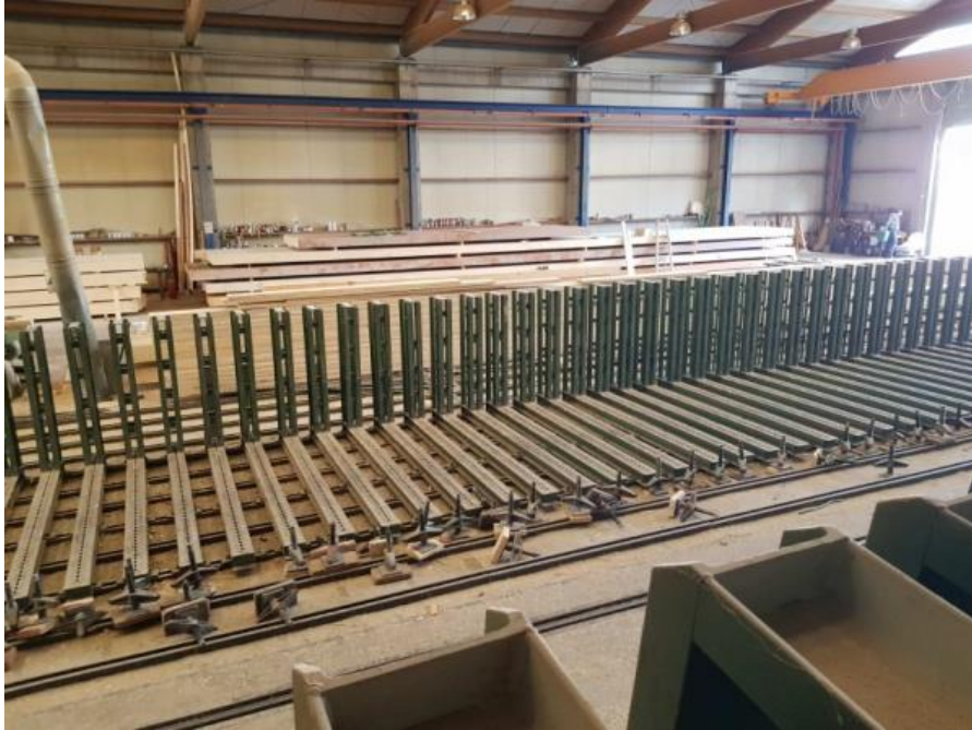
Figure 5a: Press of a length of 30 m.
